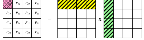
Figure 2: Matrix distribution example. In a 4 \times 4 process grid, process P_{00} needs blocks of matrix A from P_{00} , P_{01} , P_{02} , and P_{03} , and blocks of matrix B from P_{00} , P_{10} , P_{20} , and P_{30} .
