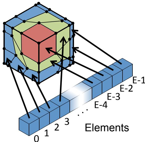
Order of values (nodes, elements, etc.) in arrays need not correspond to any ordering of simulated space.
